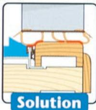
"Fin" designs will often leak when under pressure. Leading Edge Bulb Door Bottoms are superior to "fin" designs in that they have more surface contact with the threshold cap.
