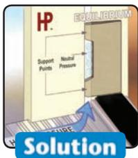
Air pressure increases on the exterior side of door system causing water to flow up the interior column of the weatherstripping. The HP Corner Pad™ blocks water under these conditions, and the result is improved performance.
